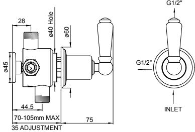
Concealed diverter with 1 inlet 2 outlets and lever or crosstop handle
