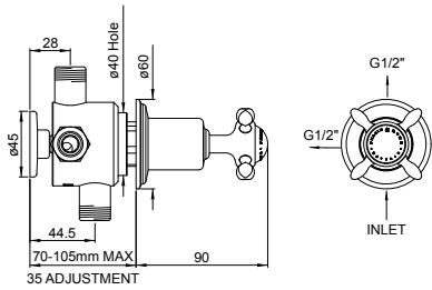
Concealed diverter with 1 inlet 2 outlets and lever or crosstop handle with shut off
