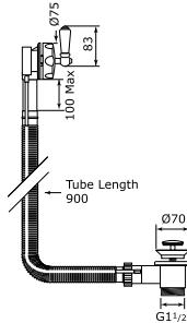
Combined pop-up waste and overflow with concealed pipes – 1200mm
