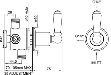
Concealed diverter with 1 inlet 3 outlets and lever or crosstop handle
