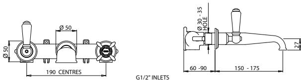
Three hole deck mounted basin mixer with pop-up waste, low profile spout and lever or crosstop handles
