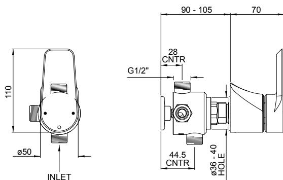
Concealed diverter 1 inlet 3 outlets with lever handle
