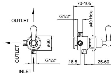
Concealed diverter with 1 inlet 2 outlets with lever handle with shut off
