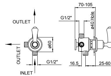
Concealed diverter with 1 inlet 3 outlets with lever handle
