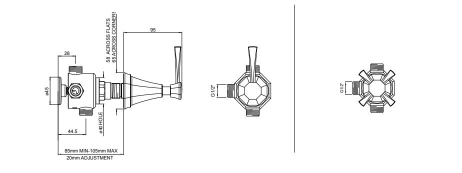
Concealed diverter 1 inlet 3 outlets with lever or crosstop handle
