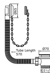
Combined pop-up waste and overflow with concealed pipes – 900mm
