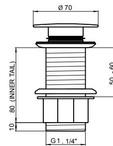
1 1/4" Basin waste metal plug stay & chain, 60mm diameter flange, 85mm tail
