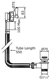
Bath waste and overflow with exposed pipes
