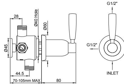
Concealed diverter with 1 inlet 3 outlets and lever handle
