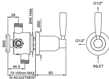
Concealed diverter with 1 inlet 2 outlets and lever handle with shut off
