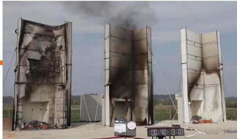
Sample 1 Sample 2 Sample 3 EPS EPS con fascia taglifuoco in MW Mineral insulation
